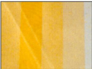
**Waviness OR Corrugation in the seam / weld area** - As the fabric rolls up along the roller tube on the awning the seams will roll up with more accumulated material than the areas surrounding it. This difference in thickness may cause the fabric to wrinkle slightly around the seams. This may affect one seam but not the seam next to it.
