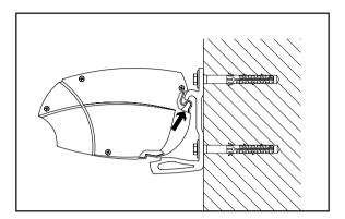
...push back and then let the awning down. Once the awning has been hooked in properly, it will support itself, but it still needs to be secured.
