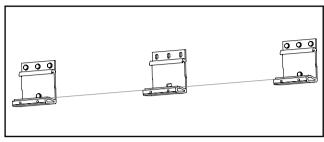
...then align the brackets exactly using a spirit level.
