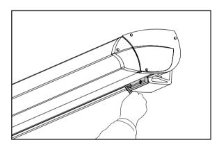
Now insert the Allen screws to fix the console closing parts to the brackets and tighten firmly with the Allen key (6 mm). This secures the awning and prevents it from falling down.
