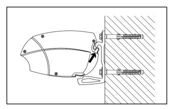
Tilt the awning upwards slightly and hook into the bracket from below...
