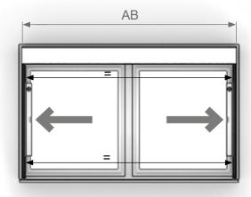
System must be square and diagonals must be equal!!
