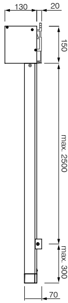
Optional face fix bracket for headbox
